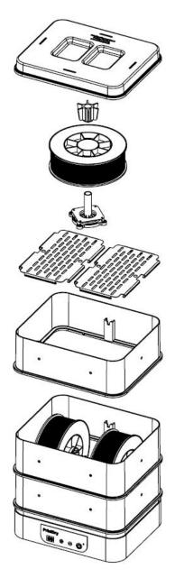
Fig.9 The use of an optional 3rd chamber kit
