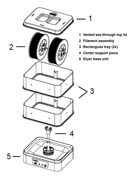
Fig.4 PrintDry Filament Dryer
