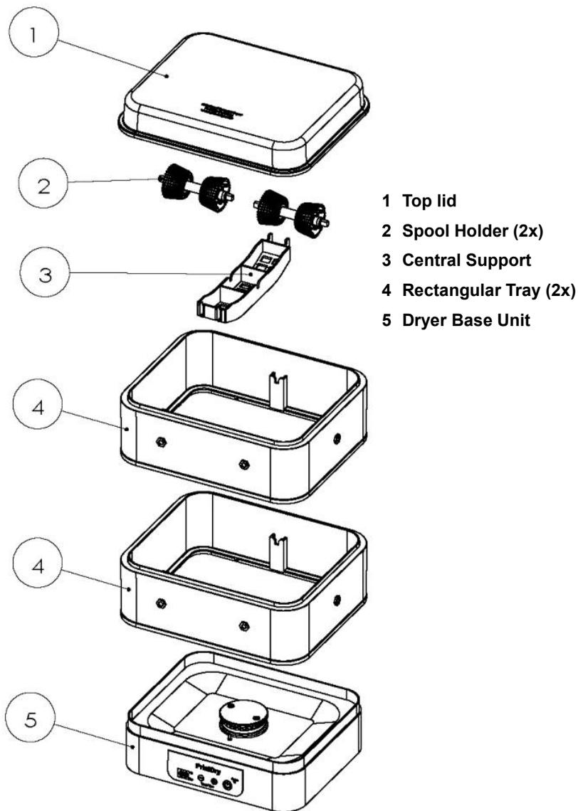
**Fig.1 PrintDry Filament Dryer**
