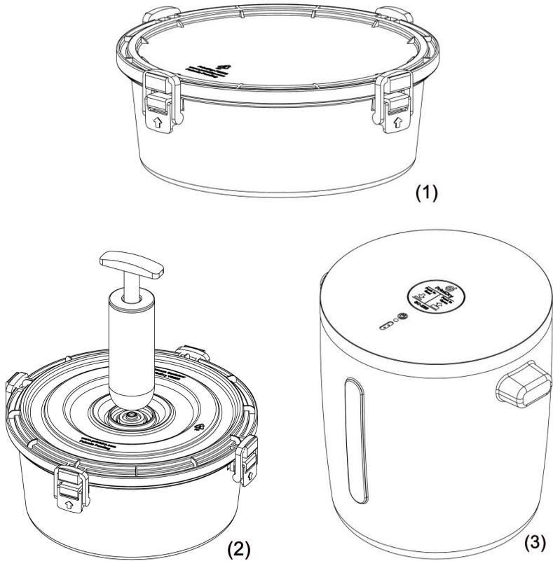
**Fig.4 Optional Filament Storage:** (1) regular filament container; (2) vacuum sealed filament container; (3) smart filament container.
